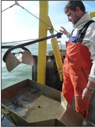
The Van Veen grab on the deck platform
